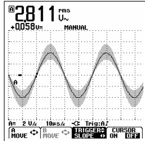
Figure 2-12. Displaying the Envelope of a Waveform
