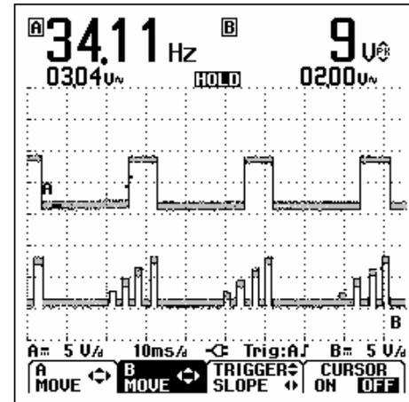
Figure 2-8. Hz and V<sub>pp</sub> as Main Readings
