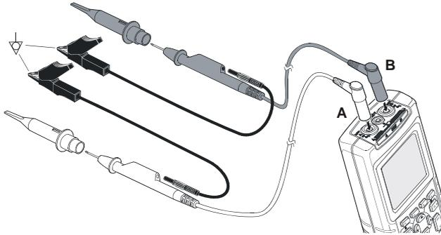
**Figure 4-1. Fieldbus Measurement Input Connections**
