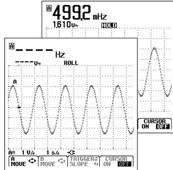
Figure 2-14. Recording Waveforms over Longer Period of Time
