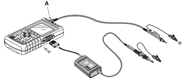
**Figure 2-16. Isolated Triggering**
