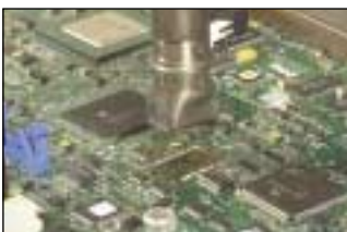
Step 1: Hot air is directed onto the leads of the QFP component.
