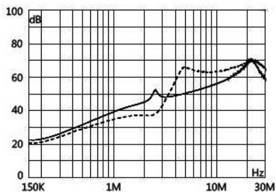
It is tested on empty load and 50Ω ( — common mode — differential mode )
