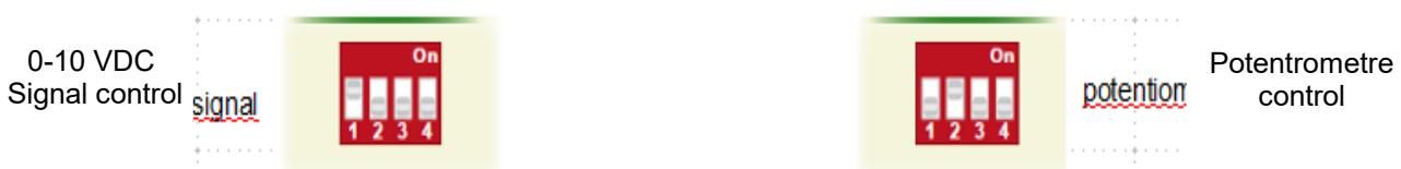
**Minimum setting :** The potentiometer as "MIN LEVEL ." It allows, through its regulation, to adjust the minimum point of activation of the load.
